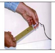
9) Attach 2-pin connector to FloodStop water/leak sensor.
