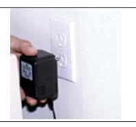
11) Plug power adaptor (transformer) into a standard 120 VAC household receptacle.
